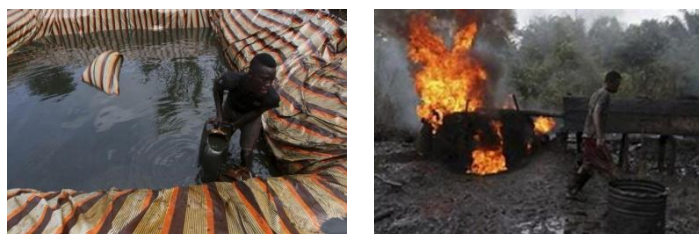
Fig. 1: (a) Illegal Refineries storage pit exposed to weather. (b) Billowing fire for heating up crude oil not far away
