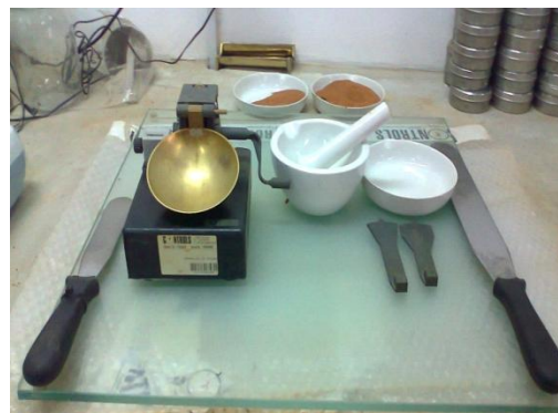
Equipment for Atterberg's limit test.
