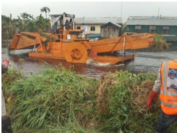
Plate 2: Manual and mechanical removal of water hyacinth and other obstructive aquatic weeds
