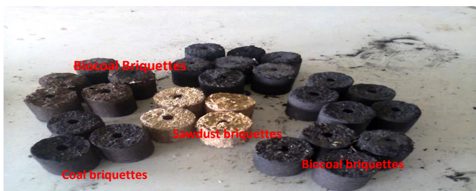
Plate 3: Samples of coal, sawdust and biocoal briquettes
